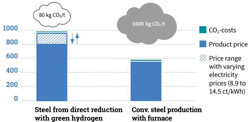
There are two different processes for steel production (direct reduction or via furnace). Because the direct reduction process with green hydrogen is still in development, this concerns our own estimate.
