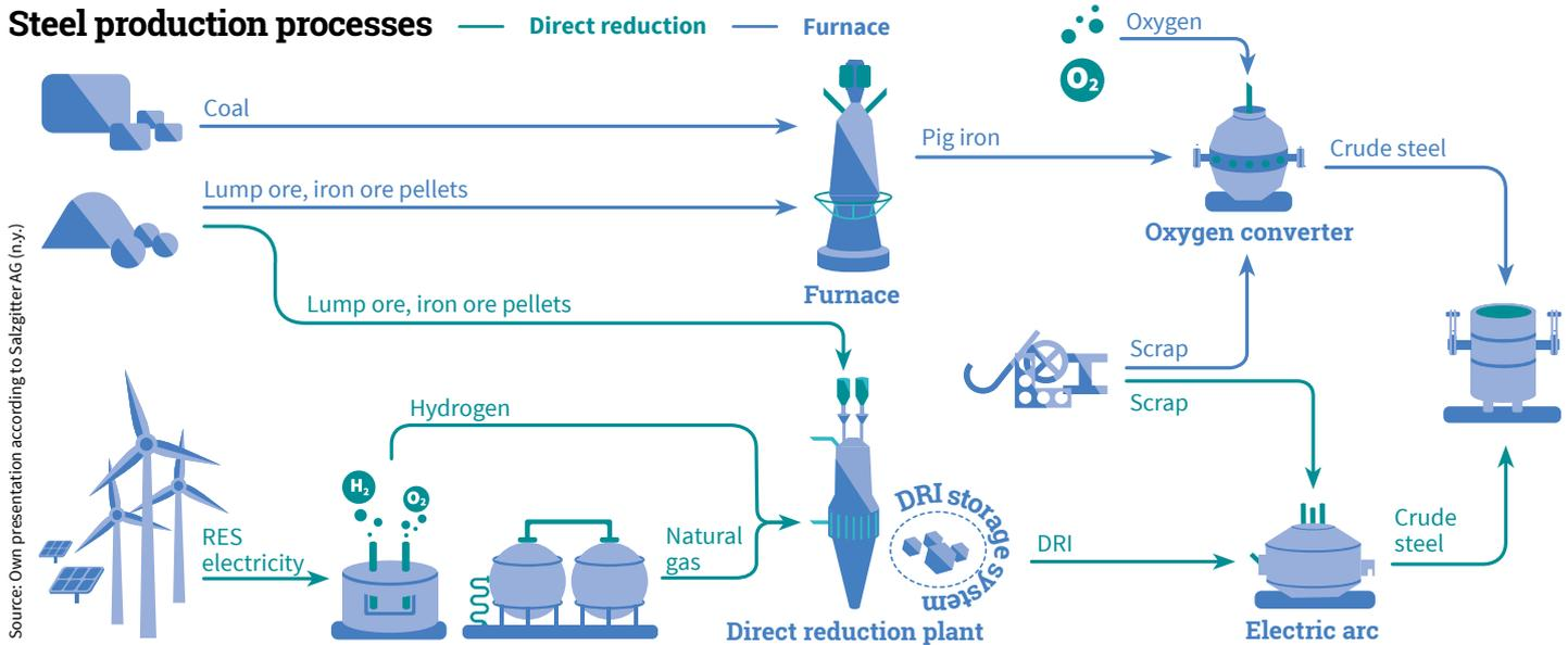
In the direct reduction process, with the aid of natural gas and/or hydrogen, iron ore is reduced to iron sponge (direct reduced iron, DRI), which can then be further processed in the electric arc furnace. The hydrogen used in the direct reduction
